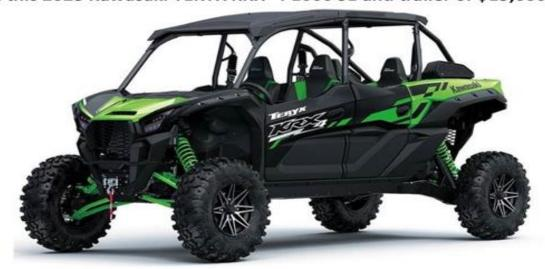
The TERYX has a 999cc, 4 stroke, DOHC, liquid cooled engine, automatic CVT transmission, belted seating for 4, 31x10 tires, a multi-function digital meter with bar-style tachometer, digital speedometer, bar style fuel gauge, gear indicator, odometer, clock, driving mode indicator, and much more.
