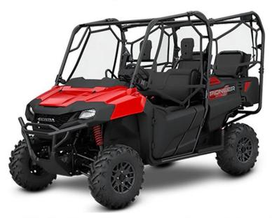
The Pioneer has a 675cc liquid cooled engine, automatic transmission, belted seating for 4, the rear seats fold down to create a cargo box.
